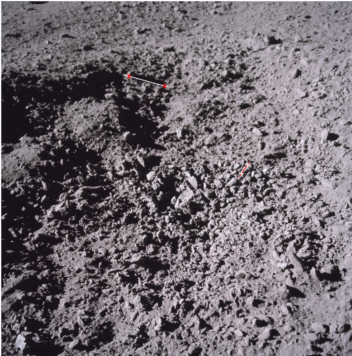
Fig. 30. To determine the orientation of the rock sample 70019, shown at middle right by the red line with white crosses, a shadow line was selected at upper middle left from a rock with straight edges raised high enough to cast shadows as unobstructed as possible. These two lines were transferred to the 3D model. The orientation of the shadow line is the solar azimuth. The orientation of 70019 is that angle plus the measured angle between the shadow line and the rock sample line. Its inclination, or slope, is that of the red line with respect to the x,y plane of the model. (NASA photo AS17-145-22189).
